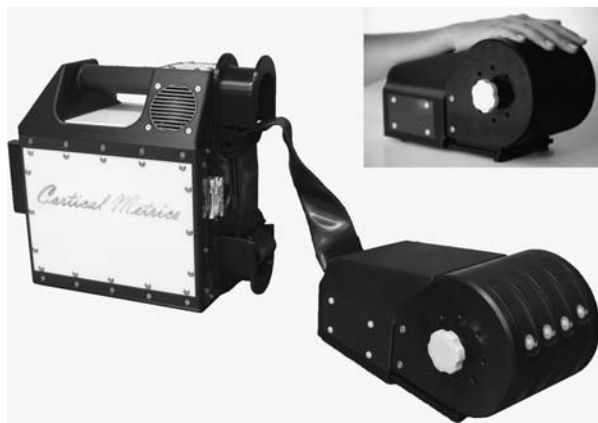
FIGURE 1. Images of the multisite vibrotactile stimulator. Stimulators are positioned by rotating each of the 4 independently positioned drums to maximize contact between fingers and the stimulator tips. During an experimental session, the patient was seated comfortably in a chair with the right arm resting on the arm rest attached to the head unit of the stimulator. Index and middle finger were positioned for D2 and D3 stimulation.
