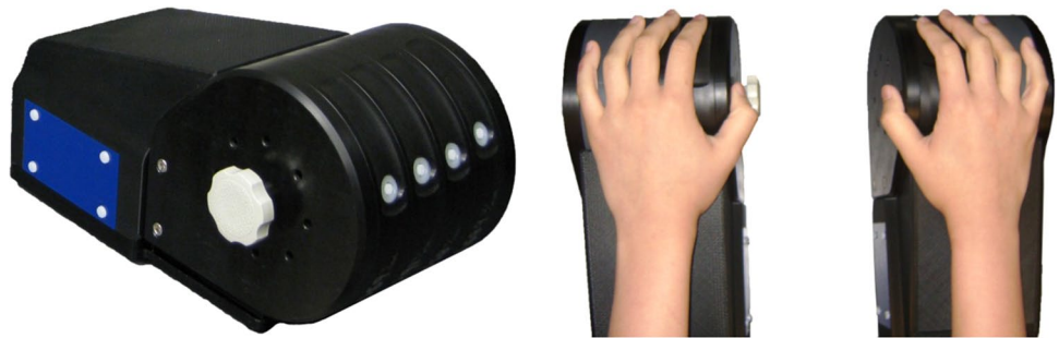
Fig. 1 Cortical metrics (CM-5) stimulator. Left and right hands were positioned on two separate head units for the bilateral protocols. The device cabling was modified to simultaneously deliver coordinated stimuli to pairs of digits on two hands (left, attended; right, unattended)
