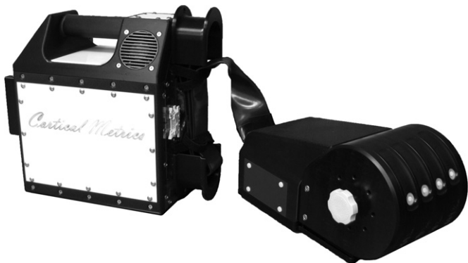
Fig. 1. Four site vibrotactile stimulator. Each of the four probe tips is positioned by rotating the four independently positioned drums to maximize contact between finger pads and the stimulator tips. During an experimental session, subjects were seated comfortably in a chair with their arm resting on the arm rest attached to the head unit of the device. Digits D2 through D5 were then positioned for vibrotactile stimulation.
