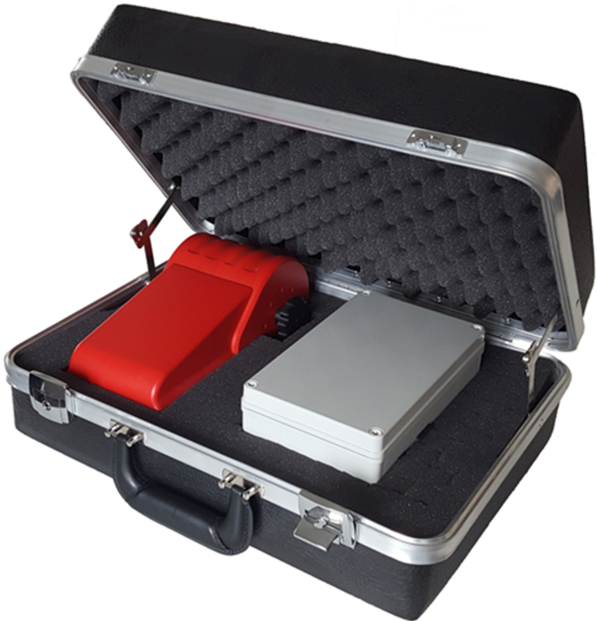
Figure 2. Complete magnet compatible stimulator system with electronic housing. Electronics are connected via a shielded cable that reaches from outside the room housing the imaging system to the MRI or MEG.
