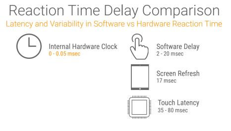
driver is polled by the CPU. This introduces a minimum of 35 ms latency in the reaction time measurement. All of these problems are inherent to visual reaction time tests, there is no way to account for the delays with software.
