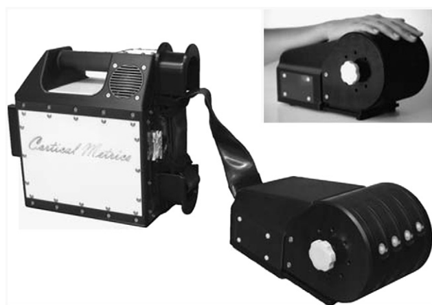
Fig. 6 – Four site vibrotactile stimulator. Each of the four probe tips was positioned by rotating the four independently-positioned drums to maximize contact between finger pads and the stimulator tips. During an experimental session, the subjects were seated comfortably in a chair with their arm resting on the arm rest attached to the head unit of the device. Digits D2 through D5 were then positioned for vibrotactile stimulation.
